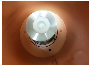
The ceramic SAGe well-detector used for measuring Hartlepool filter samples
