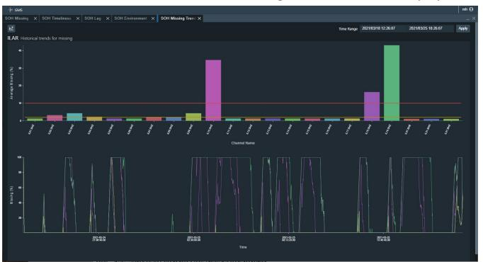
In this view of the SOH Missing Trends Display, the Average Missing data percentage is shown for each channel for the Time Range selected. The lower panel shows a trend plot for each channel, with colors matching the upper display.
