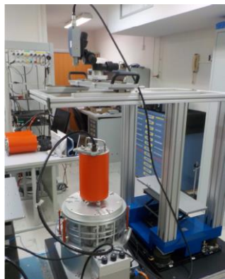
Calibration of GS13 vertical axis on shaking table
