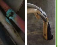
Examples of cable isolation failures due to missing strain releif and grommets when passing cables trough a steel enclosure. Sun, heat and small movements creates the broken insulation, leaving the copper exposed, corroded and creates both an electrical hazard as well as a fire hazard! IMS/MFS C. Johannsen, S. Stefanova, P. Yao
