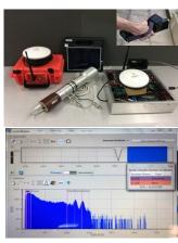
Signals are fed directly into electronics, replicating rad source spectra and encounter physics (e.g.,  $1/r^2$ ...)
