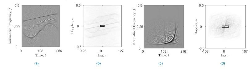
Figure 2: WVD and its respective AF of: (a),(b) z<sub>S</sub>; (c),(d) z<sub>r</sub>. The automatically selected CS-AF area has been marked by a rectangle.
