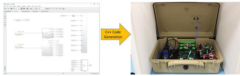
MatLab Simulink model and code used to generate C++ Code to run on sensor platform
