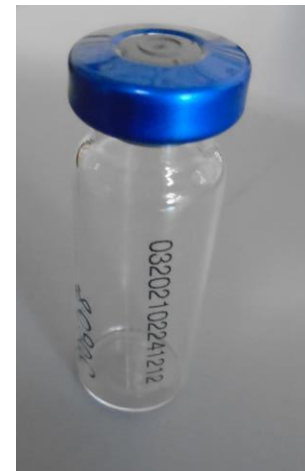
Fig. 2. Glass vial containing radioxenon sample prepared by Seibersdorf laboratories, received by GBL15.
