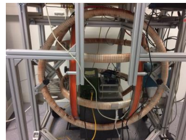
Typical magnetic sensitivity : ~100 nrad/s / Gauss
