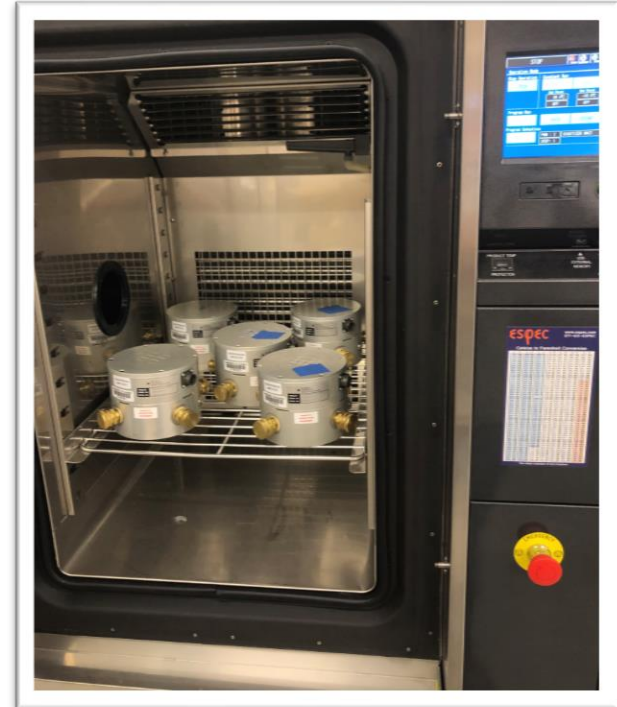
Sensors in thermal chamber for temperature soak
