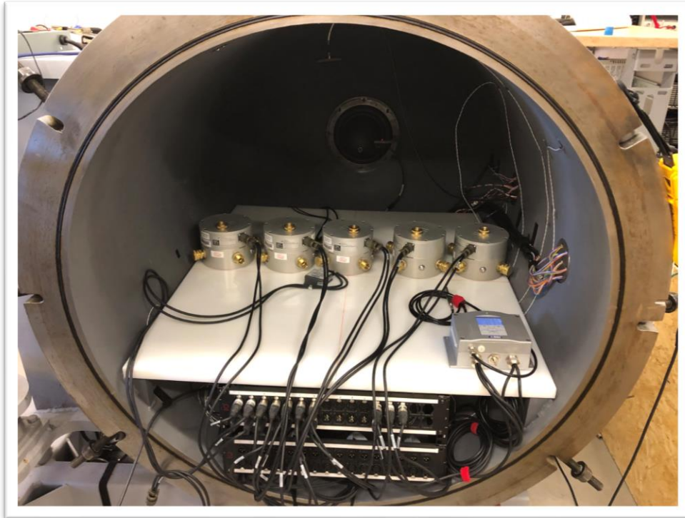
Sensors in infrasound isolation chamber
