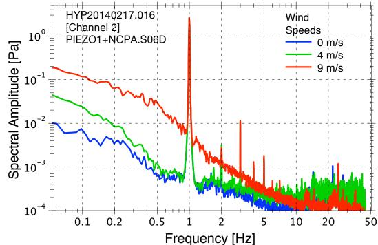
Measurements over three days able to go from 0 m/s to as high as 9 m/s! Amplitude of 3 Pa—newer systems ≥ 10 Pa.
