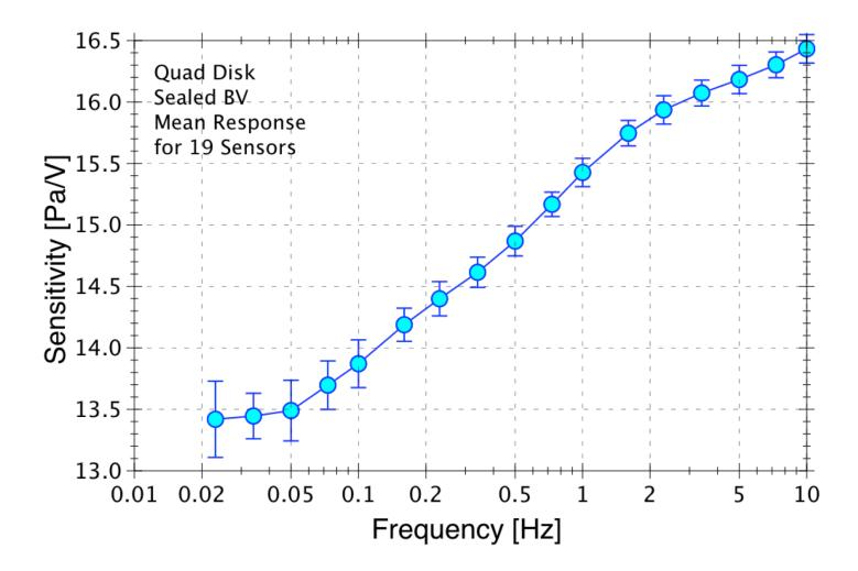
Mean & Standard Deviation of Frequency Response over 19 Sensors
