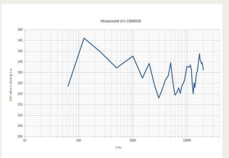
Electrodynamic moving-coil underwater speaker, two opposite 18 cm dia. carbon fibre membranes
