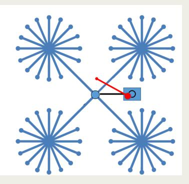
On-site calibration uses ambient signals for a calibration by comparison with the calibrated (primary & secondary) reference sensor.
