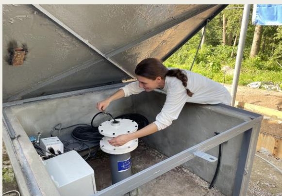
Seismometer installation AS118, Puerto la Cruz, Venezuela
