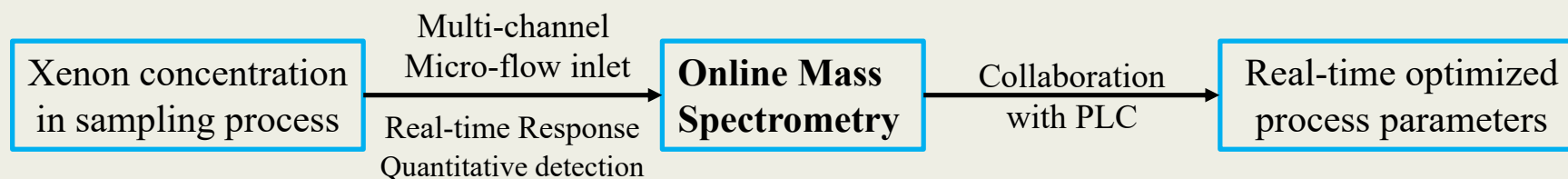
Fig.7 Schematic diagram of the intelligent sampling process for atmospheric radioactive xenon based on online mass spectrometry
