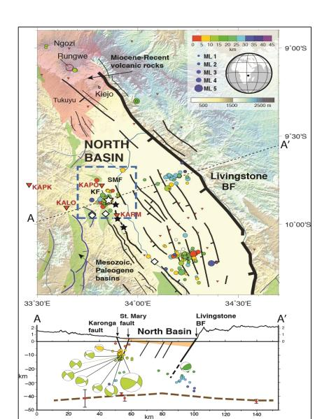
Map of North Basin of the Malawi rift zone. The white star indicates the 2014 M<sub>w</sub>5.2 Karonga earthquake that occurred in the hanging wall of Livingstone border fault. Inverted triangles are seismic stations. From Ebinger et al., 2019
