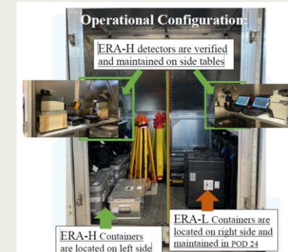
Example of operational configuration: flight POD 21 (ERA) ready to support Inspection Team Functionality (ITF) in 24 hours after deployment at BoO
