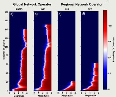
Combined probability of detection plot for all distance ranges a-b) Are stations that are operated, maintained and often picked by an organization that focuses on detecting seismicity around the world. c-d) Are stations that are operated and maintained and picked the most often by organizations that are focused on their specific country or region. You can see how these different focuses effect reported detection capability.
