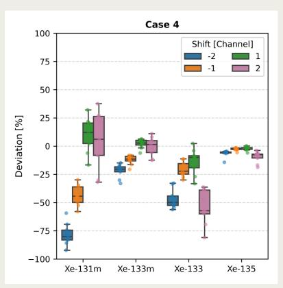
Case 4: The most complex mixture showed the broadest range of deviations. Xe-135 was the least 1.0) affected isotope, whereas Xe-131m exhibited extreme negative deviations under -2 channel shift. The relative insensitivity of Xe-135 can be explained by its larger gamma branching ratio, which reduces the influence of the calibration shift on its area estimation. In contrast. isotopes with smaller gamma branching ratios are more strongly impacted by shifts, leading to larger deviations.
