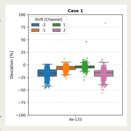
**Case 1**: Deviations were moderate compared to Cases 2 to 4. However, even a one-channel shift produced notable bias, demonstrating sensitivity to calibration even in the single-isotope case.
