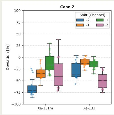
Case 2: Larger deviations were observed, in some cases exceeding -75%. The presence of both metastable and stable isotopes increased sensitivity to calibration shifts, especially for Xe-131m.
