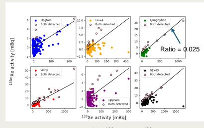
A corresponding plot for <sup>133</sup>Xe vs. <sup>133m</sup>Xe is shown above. Also here, no significant bias could be observed with increasing <sup>133</sup>Xe activities. The strongest samples all have a ratio of about 0.02, for both the array and the IMS SAUNA III. This serves as an independent check that the SAUNA CUBE units measure the same ratios as the certified IMS station.
