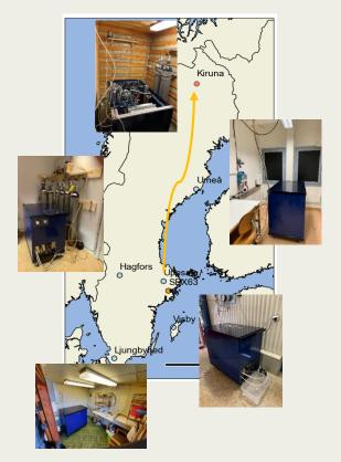
The Swedish radioxenon array (SXA) [1] is the first of its kind, consisting of five SAUNA CUBE units, each with a measurement sensitivity comparable to the SAUNA II systems used in IMS, but considerable lower cost. The size of the array is abut 950 x 450 km (see map to the left). Later, one unit was moved to the north of Sweden. The IMS station SEX63 is located in Stockholm (red dot).
