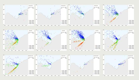
Distribution of the source locations of the detected infrasound signals by PMCC analysis (from January 01 to December 31, 2019, represented by separated panel for one month), combined by both the SYO and LNG arrays. Colors representing in right hand side for each panel correspond to the central frequency [Hz] for each detected source event.
