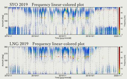
Azimuthual variations of the detected infrasound signals for whole year in 2019, for two arrays in SYO and LNG, in LHB of East Antarctica. Colors are varied on frequency ranges.
