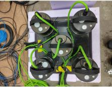
Testing of new equipment in SNSN's field lab (colocated with permanent SNSN station FIBY, ca 20km southwest of Uppsala). Huddle test to determine coherence and instrument noise. and to check overall system performance.
