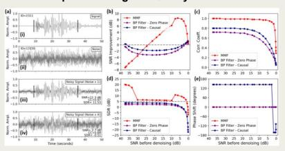
MMF is efficient for low input SNR, and significantly outperforms FF in that SNR range.
