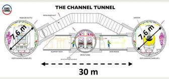
2 survey profiles across the Channel Tunnel, consisting of two rail tunnels 7.6 m in diameter and 30 m apart, excavated in chalk marl at 90 m depth. Depending on the technique, the lengths of the profiles varied.
