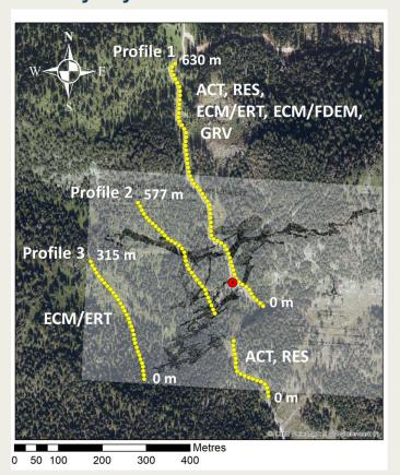
3 survey profiles over a cave system embedded in limestone with karst voids 5-15 m in diameter at depths of 40-350 m mimicking tunnels and underground cavities associated with a UNE. Depending on the technique, the lengths of the profiles varied.
