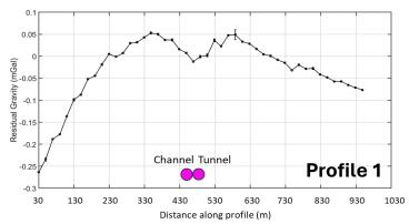
GRV results for Profile 1 showing an anomaly consistent with the Channel Tunnel target.
