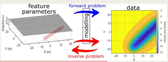
Due to the passive nature of the measurement, the signal is not attenuated or shielded by ground conditions like other geophysical techniques, and has good resolution with depth. However, due to sensitivity to vibrational noise and the need to average this out, the technique is relatively slow to acquire data, leading to high time cost, low spatial resolution, and therefore a high inspection team functionality (ITF) risk.
