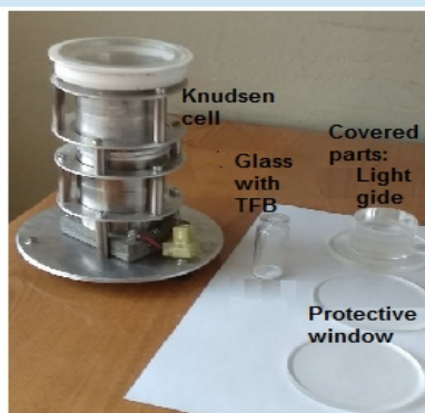
Knudsen cell, bottle with a TPB and elements to be deposited
