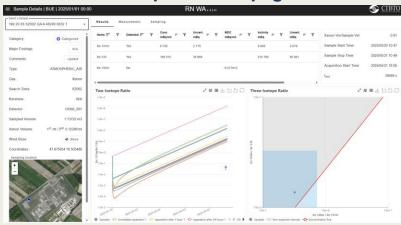
Figure 3: PaNG shows details on sample type, collection start and stop, sampling location, and radioisotope measurement results for an atmospheric gas measurement. Isotopes and ratio plots are provided here for a xenon measurement from atmospheric air.
