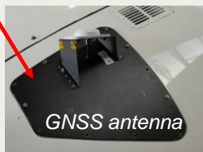
Pod with sensors installed on Bell 412 helicopter Certified aircraft engineer support is required for the installation of equipment, particularly for externally mounted devices and to access power systems
