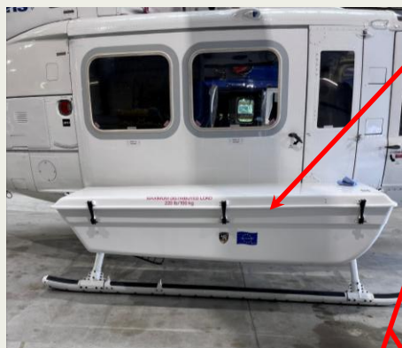
Pod with sensors installed on Bell 412 helicopter Certified aircraft engineer support is required for the installation of equipment, particularly for externally mounted devices and to access power systems
