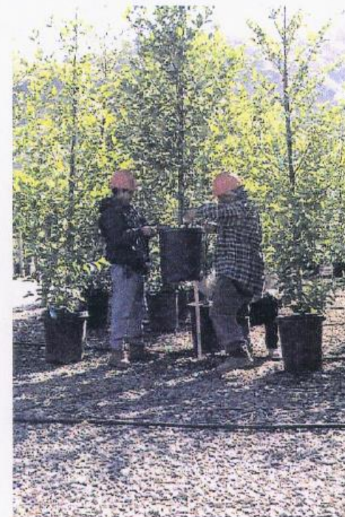
Figure 2. The pots were dropped from a measured height of one, two, or three feet.
