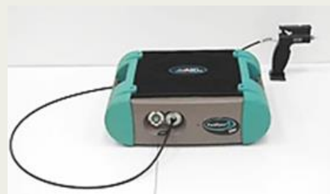
ASD FieldSpec 3 MAX spectroradiometer with PlantProbe sensorhead
