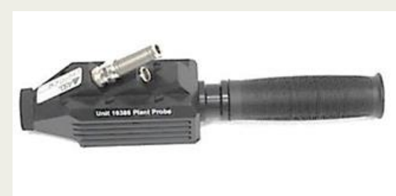
ASD FieldSpec 3 MAX spectroradiometer with PlantProbe sensorhead
