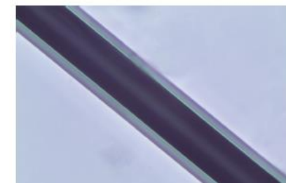
Optical microscope image of amorphous wire
