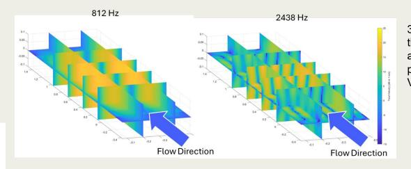
3D Model of the Acoustic Velocity in the Agglomeration System. The X, Y and Z axis are in meters and color plot is the magnitude of the Acoustic Velocity Vector (dB re 1 m/s).
