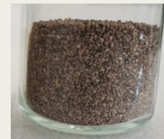
Fig. 1 – Granules of a surface treated Ag-Chabazite sample.
