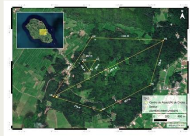
Fig. 2 - Location of IS42 and array geometry.
