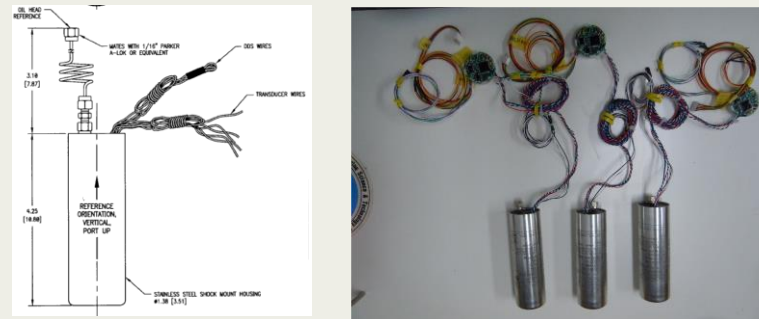
Figure 1. Drawing of the pressure gauge of Paroscientific, Inc., '410K-184' (Left), and three pressure gauges tested in the pressurization experiment (Right).
