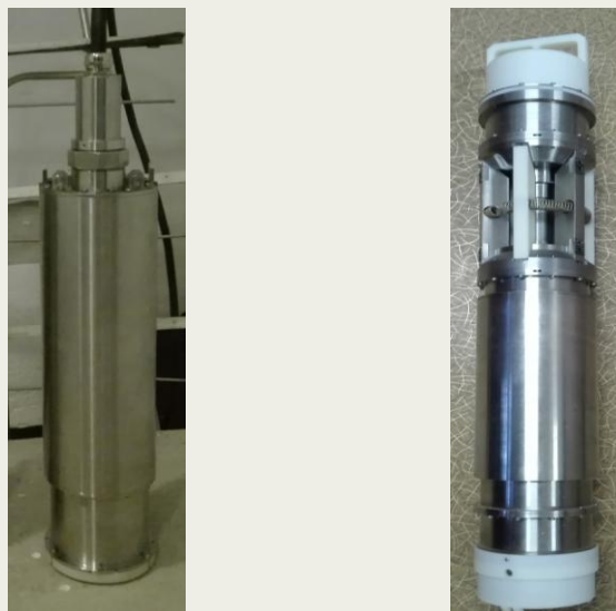
Figure 3 – Short-period vertical module, Hole-lock
