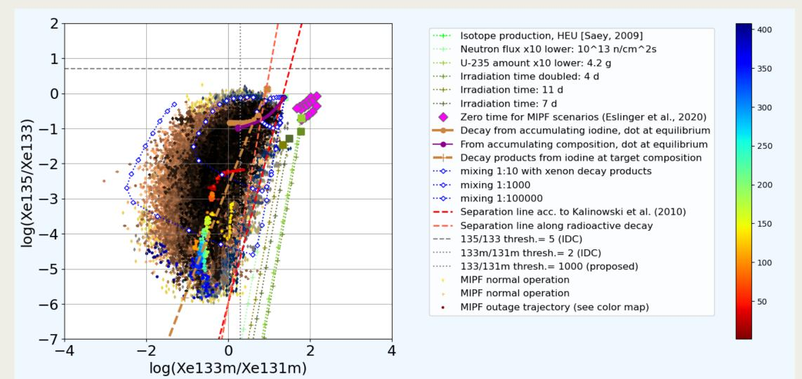
Outage time trajectory shown on top of all STAX data for a Medical Isotope Production Facility (MIPF) aligns well with radioactive decay.
