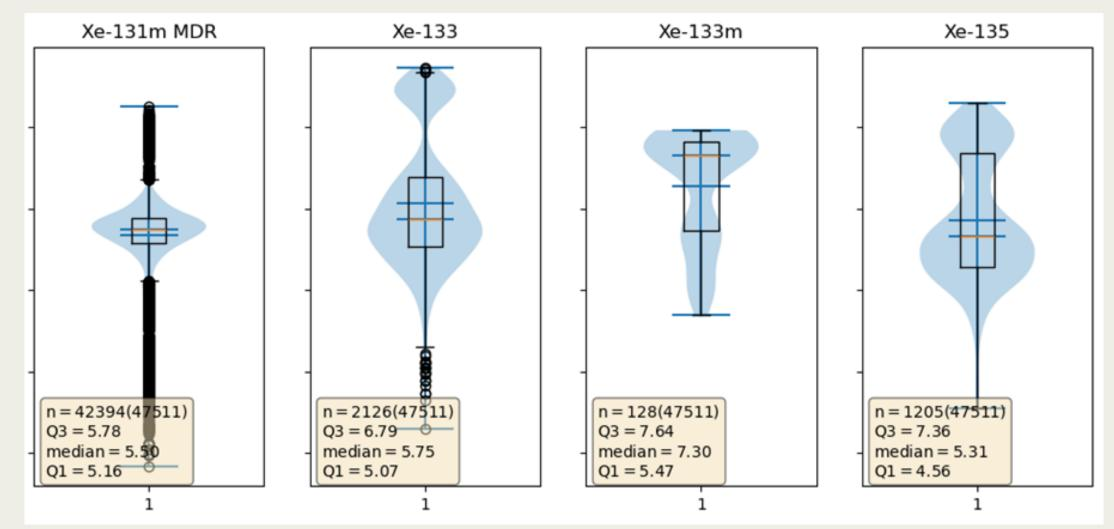
Combined violin and box-and-whisker plots showing the distribution of the logarithmic activity release rates in Bg/h of an NPP.
