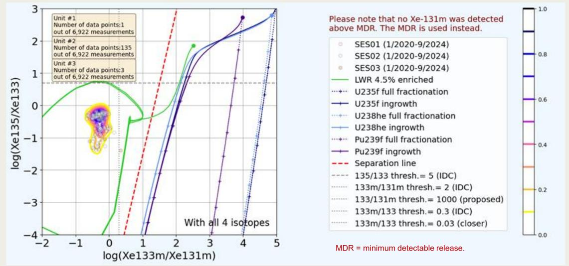
For NPPs the <sup>135</sup>Xe/ <sup>133</sup>Xe ratio is never above the IDC event screening threshold of 5, <sup>133m</sup>Xe/ <sup>131m</sup>Xe(MDR) ratio is always below 2, but the true <sup>131m</sup>Xe not known.
