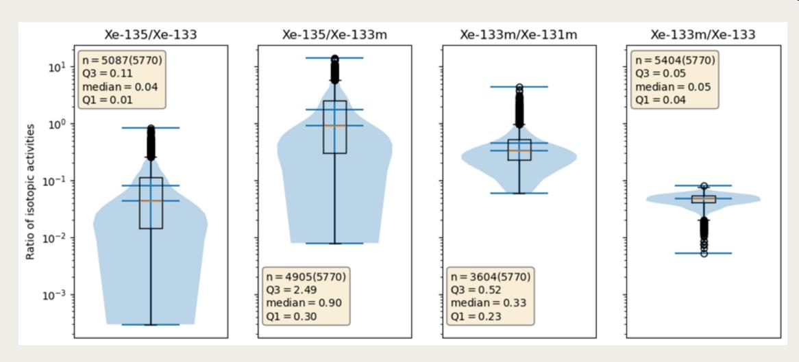
For MIPFs the <sup>135</sup>Xe/ <sup>133</sup>Xe ratio is never above the IDC event screening threshold of 5. In case of <sup>133m</sup>Xe/ <sup>131m</sup>Xe, the outliers are above the threshold of 2.
