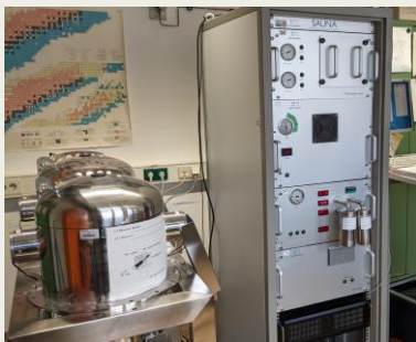
MDA Xe-133 (2 m 3 air, 24 h aq.): \approx 1 mBq Analysis of \beta - \gamma -data with openSpex
