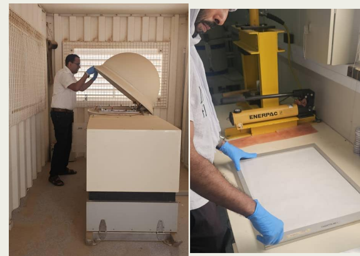
Snow White high-volume air sampler used for PM10 collection
