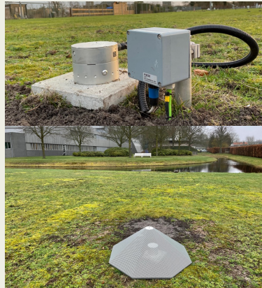
(left) Map showing the location of Dutch infrasound arrays / stations. All data is freely available via rdsa.knmi.nl and eida.orfeus-eu.org:18000 (right) Photo of an infrasound element of the De Bilt (DBN) array showing sensor and wind-noise reduction filter (dome)
