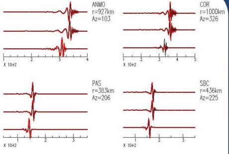
Example of simulated seismograms (dark traces) which were computed using an arbitrary solution from many that had a 98% variance reduction.
