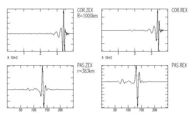
In each panel above, bandpass filtered GFs between 0.03 to 0.1Hz for 10 depths ranging between 300m to 1200m at an interval of 100m are shown on top of each other. The WUS model has a 5.5 km top thick layer. Unless the near-surface and wave-propagation paths are complex, this observation suggests no significant differences in the waveforms (may see a feeble effect in the amplitude !!!).
