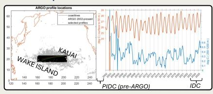
The now mature ARGO (deep-profiling floats) program provides measurement of Deep Sound Channel (DSC) temperature to constrain ocean state climate estimates. Along the propagation path from Kauai to Wake Island seasonal Ocean Atlases track the average surface layer temperature (0-50 m : red line); the temperature of the DSC (250-1250 m : blue line) corresponds to multi-year climatic events, i.e. deviations from the Ocean Atlases.
