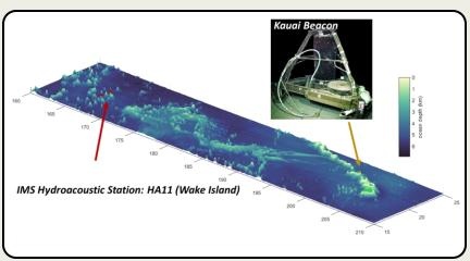
The KB is positioned 50 km north of the Hawaiian Island of Kauai, on the seafloor at a depth of 800 m. The propagation path to Wake covers 3,500 km of the Pacific Basin and passes over the undersea Mid-Pacific Mountains, which rise to within 1 km of the sea surface. The impulse energy arrives over roughly 1 second and has a characteristic twin peak arrival structure – a convenient consistent signal envelope to directly estimate the deviations in hydroacoustic travel time.
