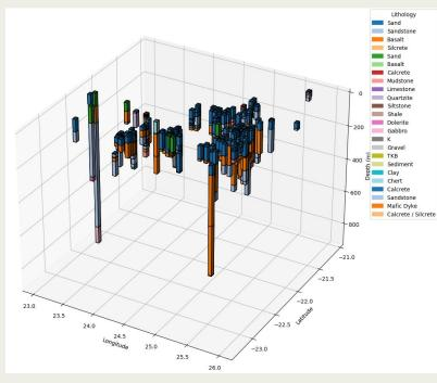
Preliminary analysis of exploration and water borehole drill logs reveals subtle but consistent shifts in lithology that may indicate the presence of faulting. While the results are not yet conclusive, the apparent offsets and changes in stratigraphy align with the orientation suggested by seismicity patterns, including the NW-SE trending fault inferred from the CKGR earthquake and aftershock distribution. Botswana
