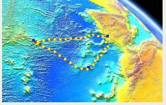
The Tam-Tam cable crossing the trench/subduction zone between Vanuatu and New Caledonia (left) to improve their telecommunications will provide valuable early warning tsunami capabilities and earthquake early warning.
