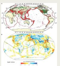
(a) Global seismic observations are largely confined to land-based sensors (green) observing arrivals from heterogeneously distributed seismic sources (red). This results in a paucity of body wave raypaths, particularly beneath the oceans, limiting fidelity of our travel-time models (b).
