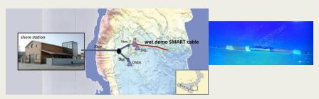
Above: An underwater electro-optical-mechanical cable runs on the seafloor from Catania harbor and splits into two branches hosting non-SMART-system geophysical, environmental, oceanographic and physics/neutrino seafloor platforms, managed by Istituto Nazionale di Geofisica e Vulcanologia and Istituto Nazionale di Fisica Nucleare, respectively. A test deployment of a SMART system with three sensors has been added to the northern branch, and began operating in December 2023.
