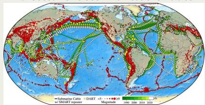
Above: Global seismicity (red) and current transoceanic cable deployments (shades of green). Cables currently cover for over 1.5 million km across the seafloors. The International Joint Task Force (JTF) for Science Monitoring And Reliable Telecommunications (SMART) Cables, a United-Nations backed initative, seeks to provide new cables and cables that replace ageing current routes, with oceanographic and geophysical sensing capability.
