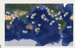
features under study such as transforms and spreading centers. Teleseismic arrivals are not reported to global archives and the 2-3 year latency for data availability contributes to their neglect. We have reviewed ~40 OBS deployments to retrieve waveforms and picks associated with large teleseismic events of interest.
