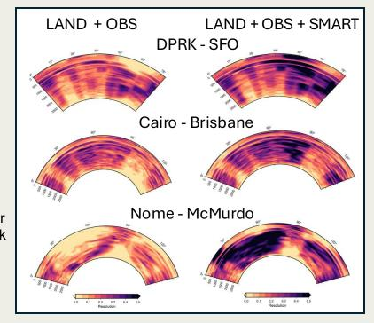
Above: model resolution gains based on addition of SMART sensors, shown for three random great circle paths through the Sandia Los Alamos 3D (SALSA3D) model (right).
