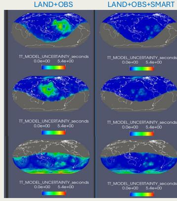
Above: Travel-time uncertainty reduction computed for land+OBS situation (left) vs. land+OBS+SMART, based on model resolution obtained for SALSA3D. Shown are TT uncertainty values for three stationis: ABJ, COLA and SBA. Note the addition of SMART sensors significantly improves TT uncertainty for all three test stations, which will directly lead to improved event location confidence.
