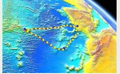
The Tam-Tam cable crossing the trench/subduction zone between Vanuatu and New Caledonia (left) to improve their telecommunications will provide valuable early warning tsunami capabilities and earthquake early warning.
