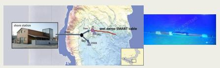
Above: An underwater electro-optical-mechanical cable runs on the seafloor from Catania harbor and splits into two branches hosting non-SMART-system geophysical, environmental, oceanographic and physics/neutrino seafloor platforms, managed by Istituto Nazionale di Geofisica e Vulcanologia and Istituto Nazionale di Fisica Nucleare, respectively. A test deployment of a SMART system with three sensors has been added to the northern branch, and began operating in December 2023.
