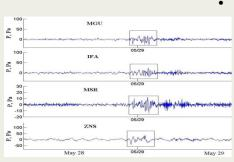
Atmospheric pressure variations on the Earth's surface, recorded on a network of four microbarographs
