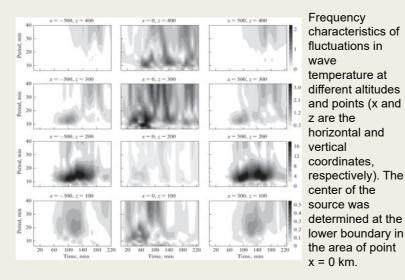
The results of the spectral analysis showed that already 30 minutes after the start of the source operation at an altitude of 100 km, waves with periods of 10-15 minutes are observed, waves with periods of 15-30 minutes are observed 120 minutes after the start of the source operation at a distance of 500 km from the source.
