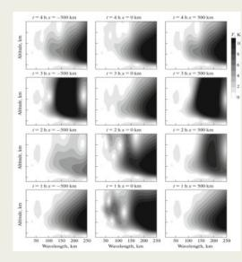
Wavelet analysis of the vertical structure of temperature disturbances. obtained with numerical calculations to distinguish the characteristics of waves in the thermosphere. The center of the source was determined at the lower boundary in the area of point x = 0 km.
