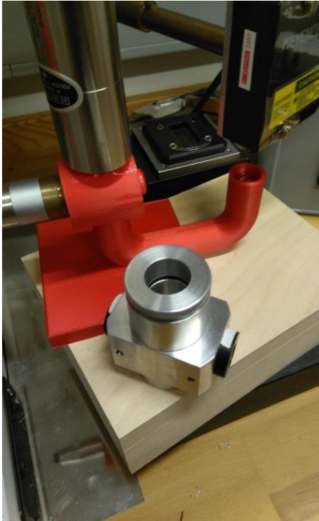
DFM manometric apparatus (dropped in Infra-AUV)
