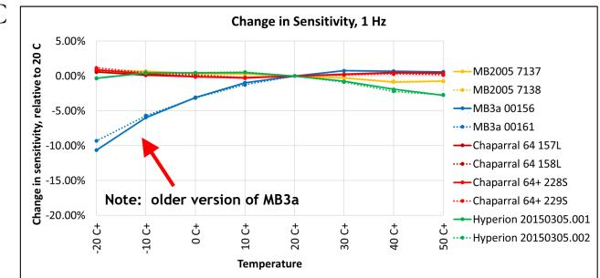
• Recent field comparison data have demonstrated issues at lower frequencies and colder temperatures.
