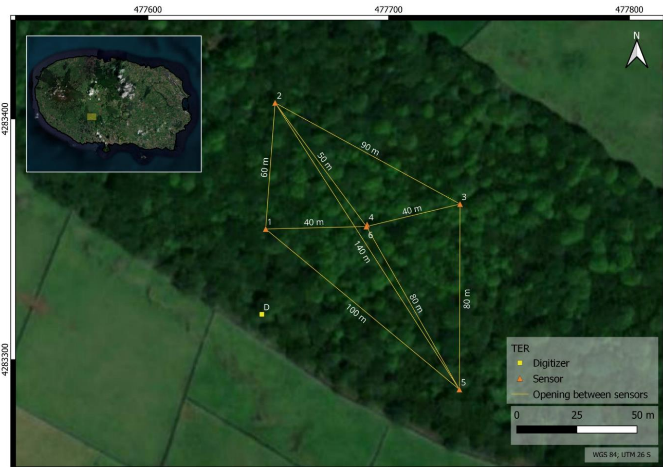
Figure 4 – Location of TER array and its geometry since 2 nd October in Terceira Island.
