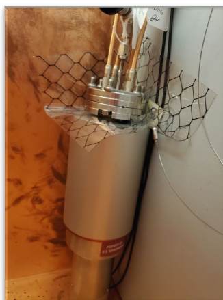
Silicon beta cell in NaI well detector.
