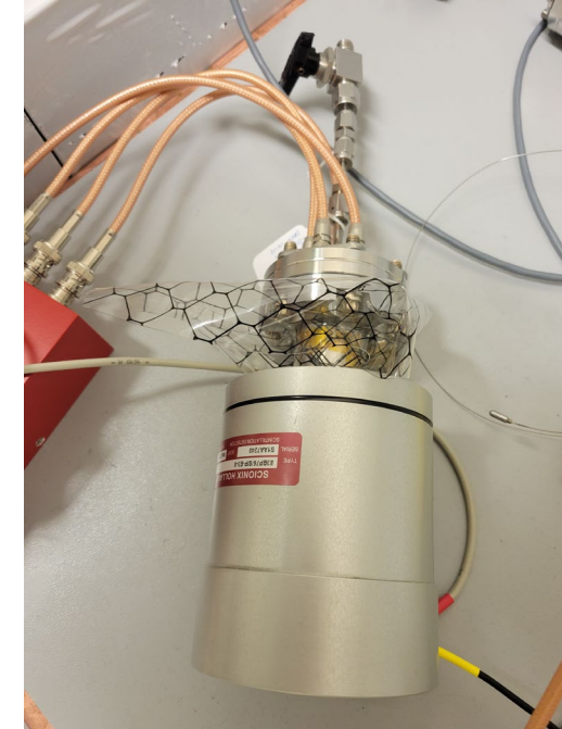
Silicon beta cell partially inserted into the SiPM based well detector.
