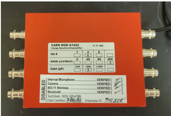
Original Caen preamplifier with 400 mV/MeV charge sensitivity
